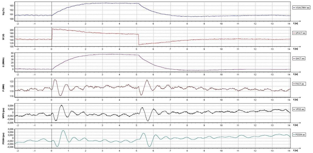
Figure 9. Generator voltage, field voltage, reactive power, active power, PSS output, integral of acceleration power signal response to  $\Delta V_{ref}=3\%$ , PSS OFF, Unit 2 Yeniköy [18]
