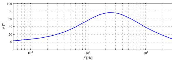
Figure 5. Phase characteristic of the lead-lag transfer function for TPP Jertovec [13]
