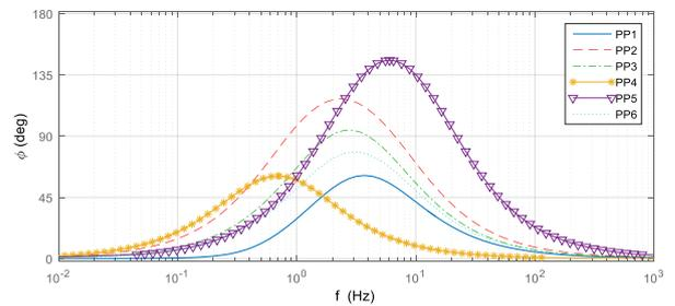
Figure 6. Example of the PSS lead-lag filter phase responses for power plants with "DRN" digital voltage regulator
