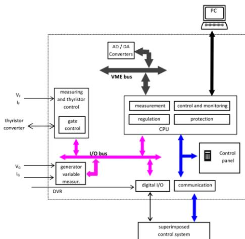
Figure 2. Block diagram of DRN structure [9]
