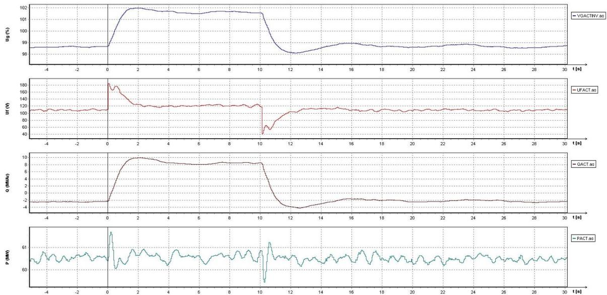
Figure 12. Generator voltage, field voltage, reactive power and active signal response to  $\Delta V_{ref}=3\%$ , PSS ON, Unit 1 Aslancik [19]
