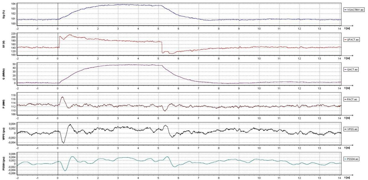
Figure 10. Generator voltage, field voltage, reactive power, active power, PSS output and integral of acceleration power signal response to  $\Delta V_{ref}=3\%$ , PSS ON, Unit 2 Yeniköy[18]
