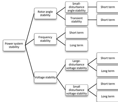
Figure 1. Power system stability classification [1]
