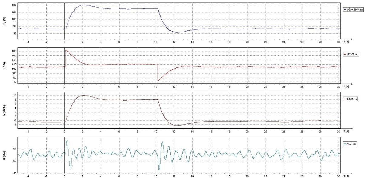
Figure 11. Generator voltage, field voltage, reactive power and active signal response to  $\Delta V_{ref}=3\%$ , PSS OFF, Unit 1 Aslancik [19]
