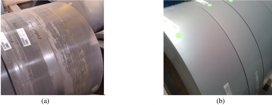
Fig. 6 Core material (a) with a low SIR value ( $8 \text{ ohm-cm}^2$ ) (b) with a high SIR value ( $60 \text{ ohm-cm}^2$ )
