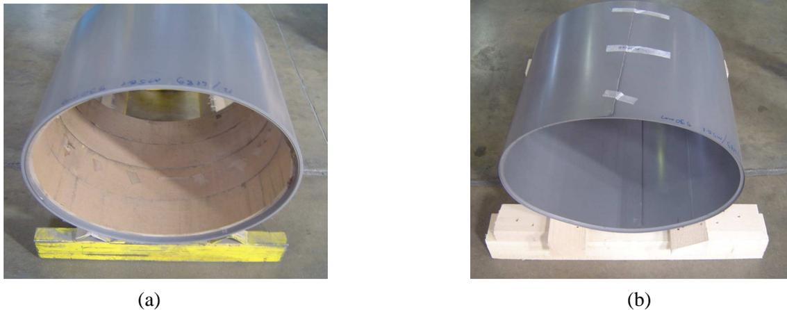
Fig. 5 Coil handling (a) with an inner guard plate (b) without an inner guard plate
